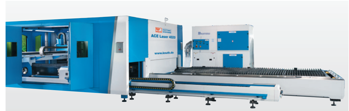
An automatic changer table system minimizes down-times
