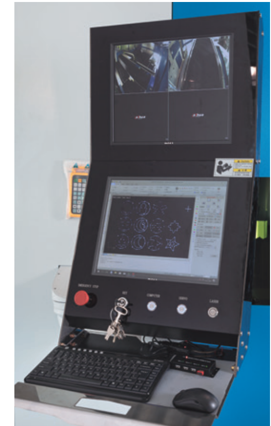
Cameras show the user real-time images of the work area and shuttle table behind the machine
