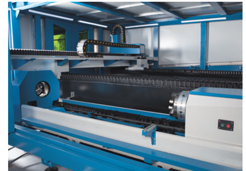
The 4-jaw chuck at the positionable headstock accepts round and square tubing
